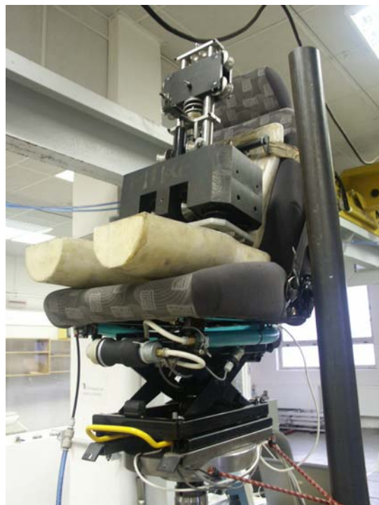
Fig. 6 – Laboratory testing of seats on simple electro-hydraulic test rig (actively suspended seat with 2-DOF dummy is shown)
