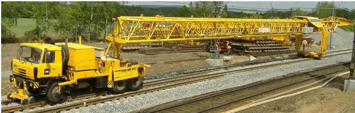
Fig. 1 - A Special Railway Crane PKP 25/20i. [15]
