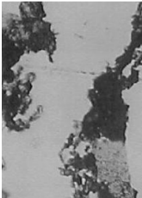
Fig. 7 - Particles of ultimate wear, they have pitting on the surface caused by repeated passage of zone of rolling contact, and they are produced at the end of fatigue wear. Magnification 500 x.
