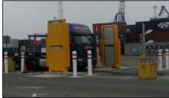
Fig. 8 – Radiation Portal Monitors installed at Port of Felixstowe (UK)
