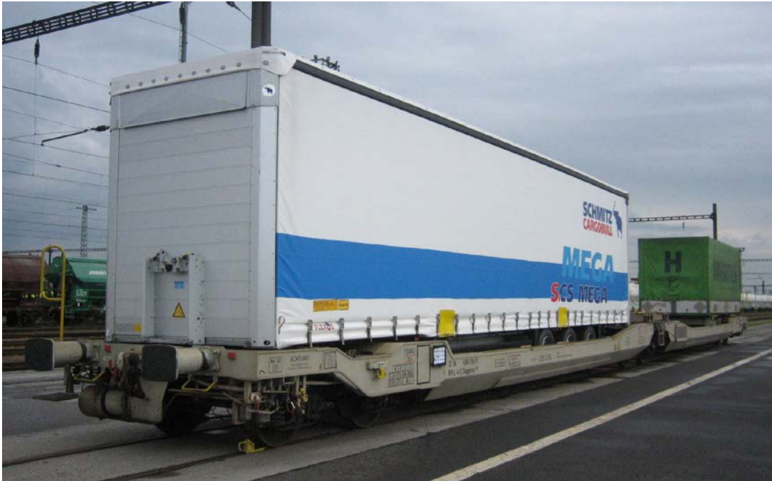
Picture 4: Wagon Sdggmrss Megatrailer with loaded cargo bulk semi-trailer S.CS MEGA and swap body C715
