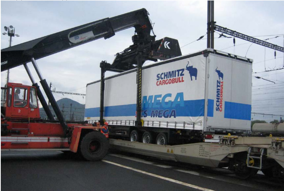
Picture 3: Loading of the semi-trailer
