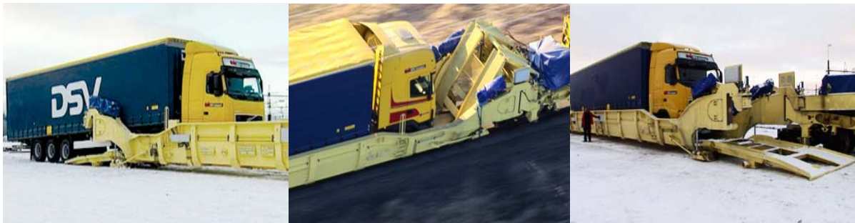
Fig. 3 - Road-set in rail waggon of system Flexiwaggon
