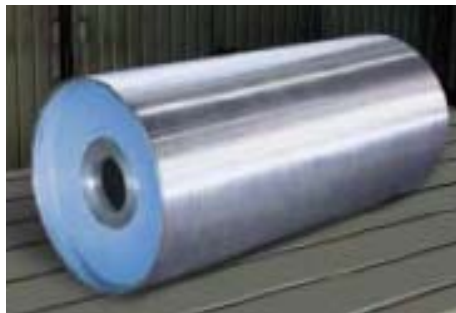
Fig. 5 - Shell of the return drum of the belt conveyor
