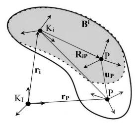
Fig. 1 - Flexible body - kinematics representation
