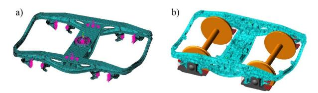
Fig. 2 - The FE model of the freight wagon bogie with interfaces nodes a) and the FMBS of the freight wagon bogie b)
