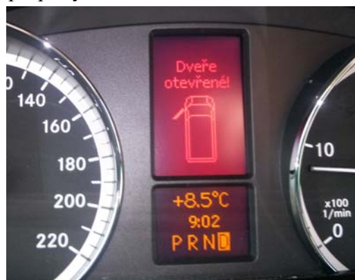
Fig. 10 - Warning that the doors are not closed properly.
