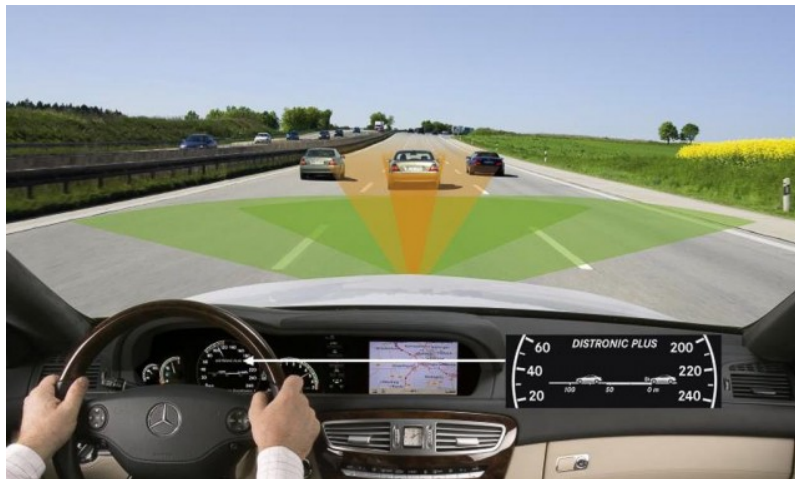
Fig. 14 - Adaptive Cruise Control (ACC). Source:
