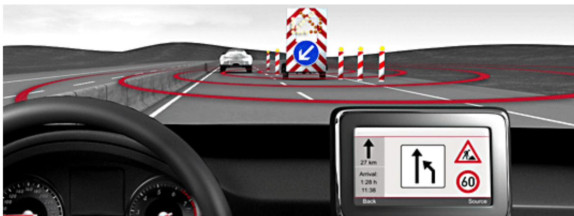
Fig. 28 - Warning the driver of the change in traffic through the system Car2Infrastructure. Source: https://vector.com/vi_car2x_de.html
