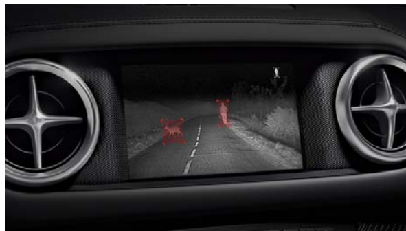
Fig. 23 - Vision Enhancement. Source: http://techcenter.mercedes-benz.com/sk_SK/night_view_assist_plus_2013/detail.html
