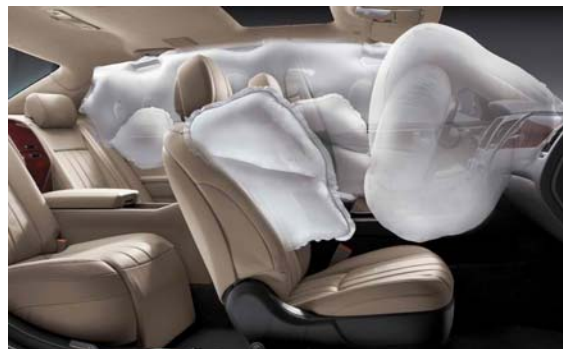
Fig. 30 - Airbags system. Source: http://www.chicagonow.com/drive-he-said/files/2014/11/Airbag_02.jpg
