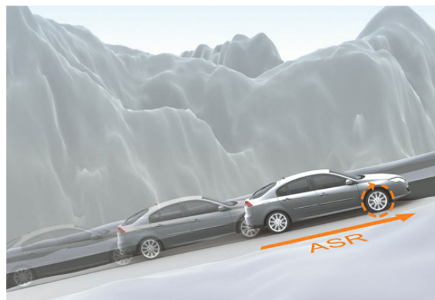
Fig. 2 - Anti-Slip Regulation system (ASR). Source: http://www.renault.cz/nove-vozy/osobni-vozy/laguna/laguna/vybava/vybava/#Bezpe%C4%8Dnost
