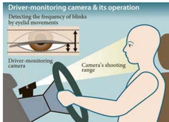
Fig. 21 - Driver Monitoring System (DMS). Source: http://web-japan.org/trends/11_tech-life/win_tec12100103.html
