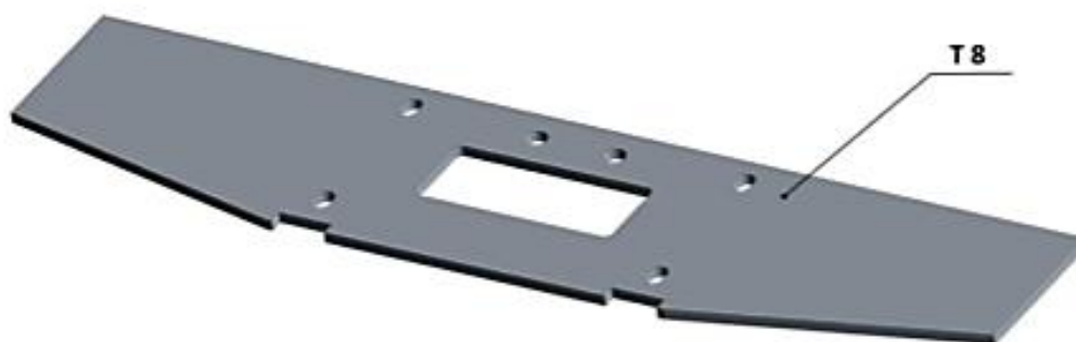
Obr. 4 - 3D model platne pre uchytenie navijaka
