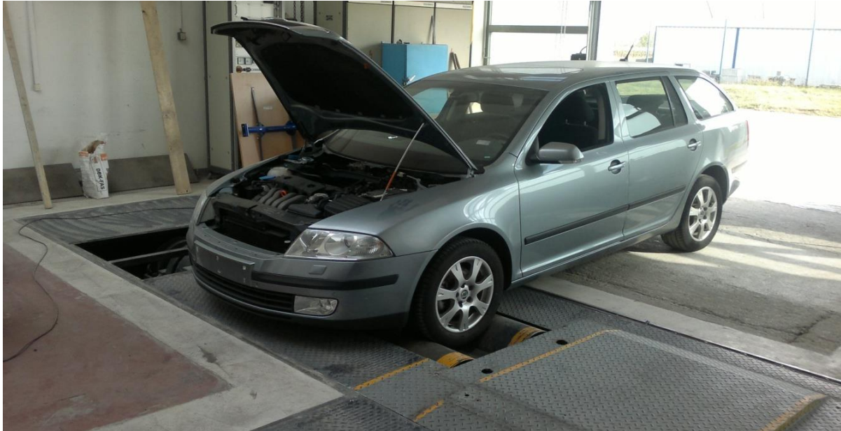
Fig. 1 – Test vehicle on the chassis dynamometer
