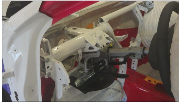
Fig. 1 – Holder + steering column of Škoda Octavia III. generation
