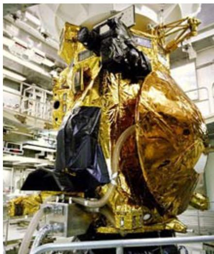
Fig. 1 - The Cassini spacecraft, with the Huygens probe seen on the right, sits atop a Titan IVB/Centaur expendable launch vehicle at the Cape Canaveral Air Station (11)
