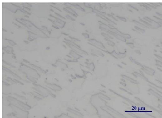
Fig. 4 – LOM image of microstructure of sample No. 3 containing lamellar phases
