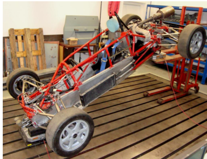
Fig. 5 – Tilting method for measurement of centre of gravity height
