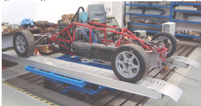
Fig. 5 – Tilting method for measurement of centre of gravity height
