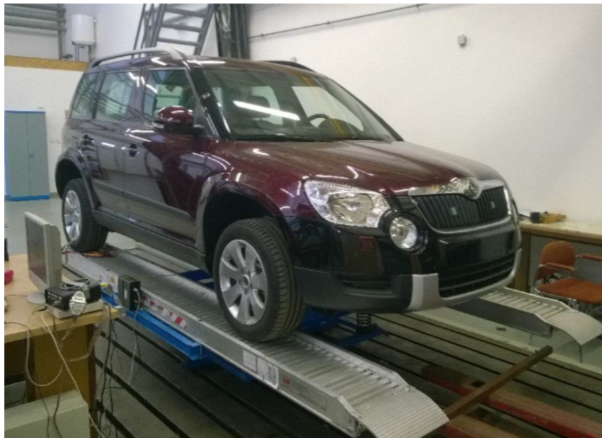
Fig. 7 – Measurement of the centre of gravity height with new method
