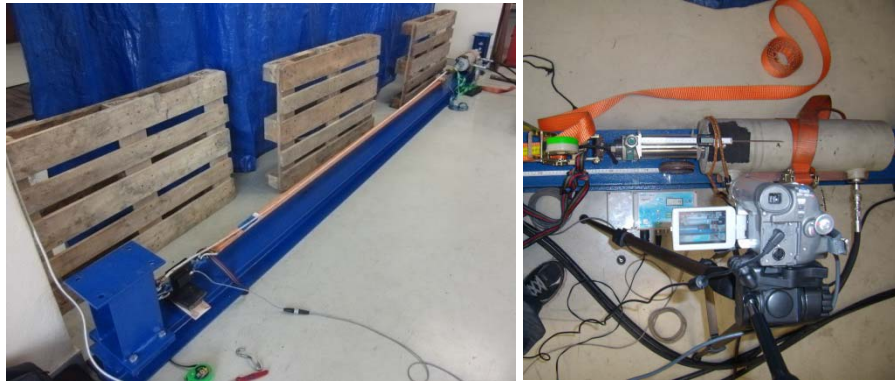
Fig. 2 - Testing stand to test tension forces in lashing straps
