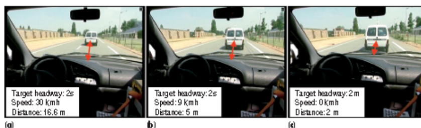
Fig. 2 – The adaptive cruise control
