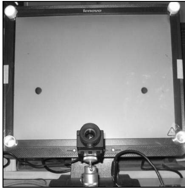
Fig. 4 - System with 4 IR sources
