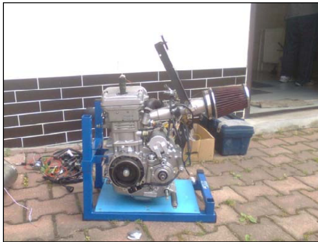
Fig. 1 - Complete MZ125 engine ready for use in autocross
