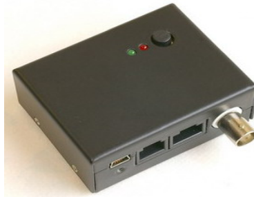
Fig. 2 - Basic flight recorder
