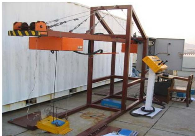
Fig. 9 - Experimental model of gantry crane
